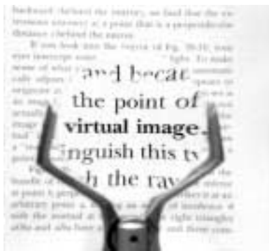
Fig. 13.3.3 - This magnifying glass creates an enlarged virtual image located far behind the printed text.
