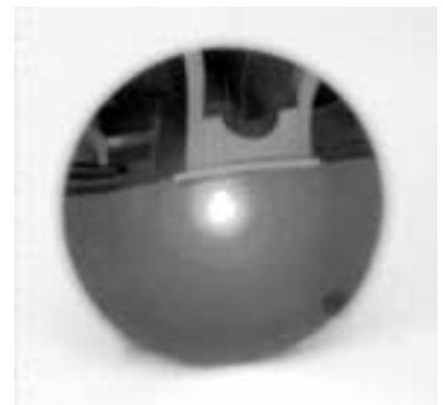
Fig. 13.3.9 - A curved mirror produces an inverted real image of a light bulb located on a table far in front of it.
