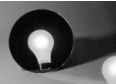
Fig. 13.3.7 - A curved mirror produces an upright virtual image of a light bulb located just in front of it.
