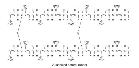
Fig. 16.3.8 - Part of a natural rubber molecule showing eight repetitions of the basic isoprene monomeric units from which it's built. The orientations of the isoprene units alternate up and down. The chains coil up randomly on their own but straighten when you stretch the rubber. The rubber reaches its elastic limit when the chains are straight.
