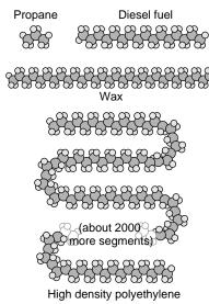
Fig. 16.3.1 - Paraffin chains are found in many materials. Each paraffin chain consists of a backbone of carbon atoms (the larger balls), decorated by pairs of hydrogen atoms (the smaller balls). A chain is terminated at each end by an extra hydrogen atom. Propane, diesel fuel, and wax contain relatively short paraffin chains while high density polyethylene, the plastic used in milk containers, contains paraffin chains of between 1000 and 3000 carbon atoms.
