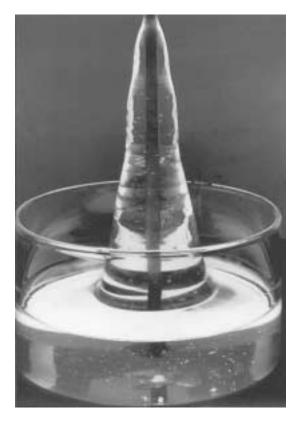
Fig. 16.3.6 - When you place a spinning rod into normal liquids, the molecules of liquid are thrown outward and move away from the rod. But in a liquid polymer, entanglements draw the polymer chains toward the rod, creating the Weissenberg effect.
