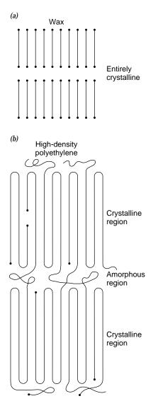
Fig. 16.3.2 - (a) Wax is a crystalline material, held together only by van der Waals forces. (b) High density polyethylene is about 80% crystalline and 20% amorphous, with entanglements helping to hold it together.
