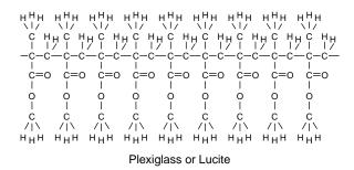
Fig. 16.3.11 - Plexiglas is long chains of poly(methyl methacrylate). These chains bind relatively strongly to one another to form a glassy, transparent material at room temperature.
