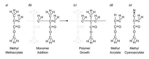
Fig. 16.3.15 - (a) Methyl methacrylate polymerizes in the presence of free radicals. (b) The free radical attacks the double bond between two carbon atoms and attaches itself to one of those carbon atoms. (c) The other carbon atom then becomes a free radical itself and begins searching for yet another monomer to attack. This process continues until a long chain is constructed. Alternative monomers include (d) methyl acrylate and (e) methyl cyanoacrylate.
