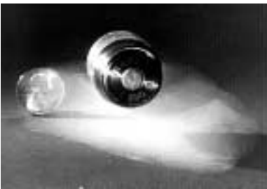
Fig. 6.5.5 - The best thermal insulators currently under study are tenuous materials called aerogels. These porous glassy structures are almost entirely air and resemble frozen smoke. There's hope that aerogels and other high performance insulators will dramatically improve the energy efficiencies of refrigerators and other machines.
