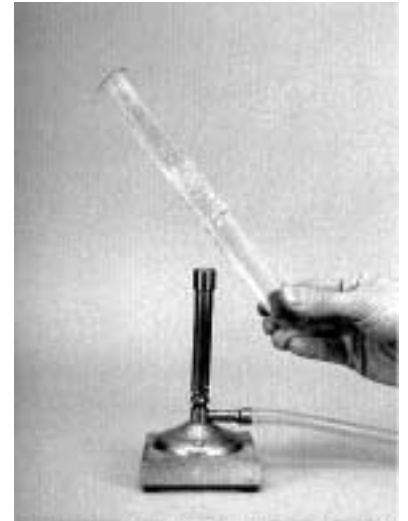
Fig. 6.5.2 - Convection only occurs if the hotter object is below or next to the colder object so that the heated fluid is able to rise. If you heat a tube of water near its top, the hot water stays near the top and the cold water remains at the bottom. Because water itself is a poor conductor of heat, the water at the top of the tube can boil while the bottom of the tube is cool enough to hold in your hand.
